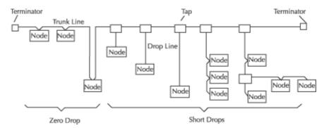
DeviceNet supports both isolated and non-isolated physical layer design of devices. An opto-isolated design option allows externally powered devices (e.g. AC Drives starters and solenoid valves) to share the same bus cable. The DeviceNet Specifications contain additional information concerning component requirements, protection from miswiring, and examples.
