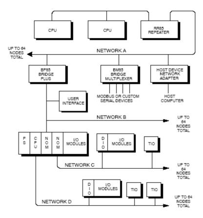
The network also provides an efficient means for servicing input/output subsystems. Modicon Modbus Plus Distributed I/O (DIO) Drop Adapters and Terminal Block I/O (TIO) modules can be placed at remote I/O sites to allow the application to control field devices over the network link.
