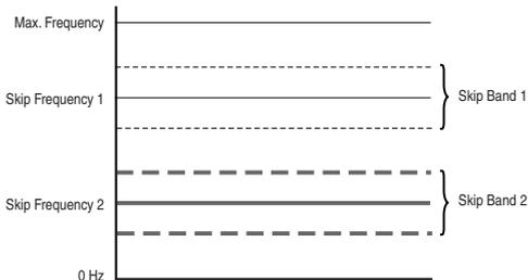
If skip bands overlap or touch, the center frequency is recalculated based on the highest and lowest band values.
