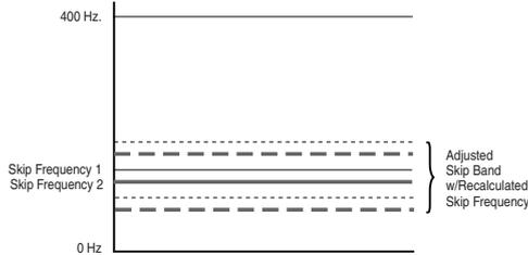
If a skip band(s) extend beyond the max frequency limits, the highest band value will be clamped at the max frequency limit. The center frequency is recalculated based on the highest and lowest band values.
