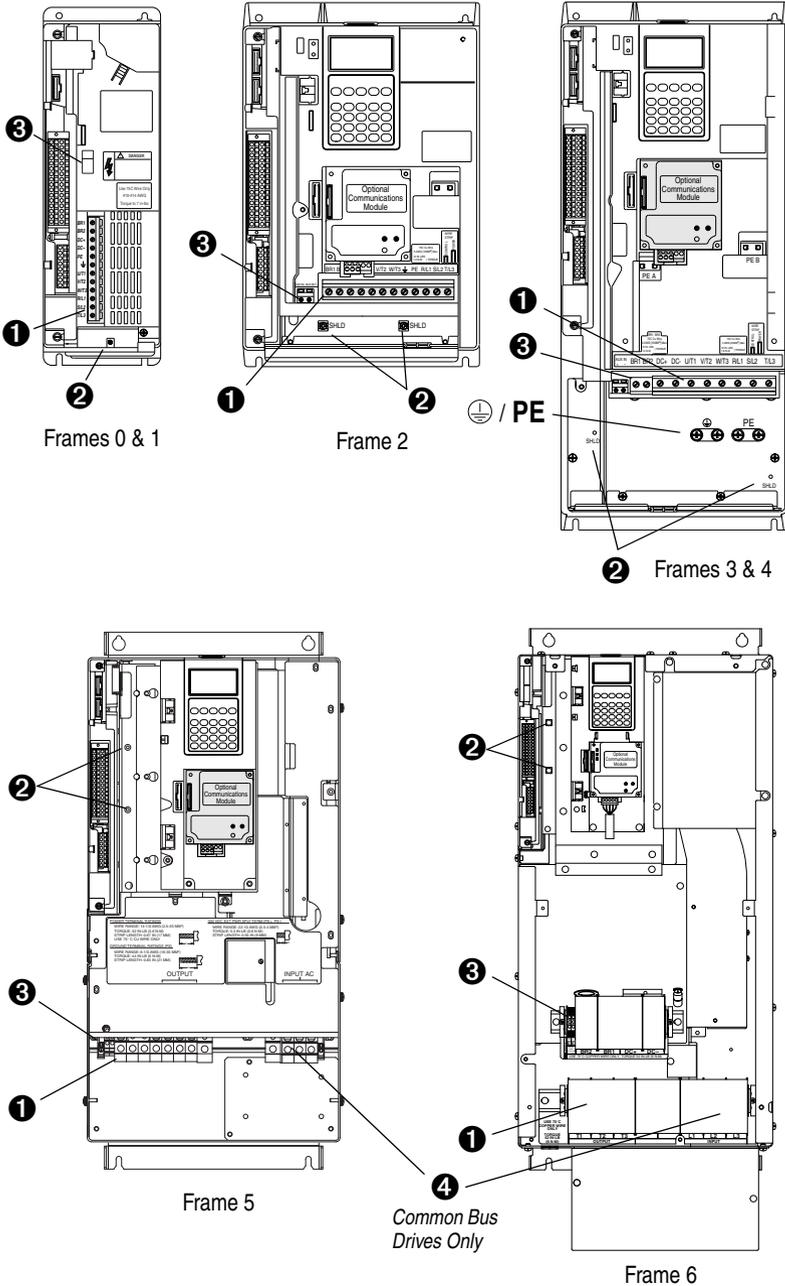
Figure 1.4 Power Terminal Block
