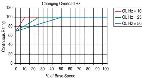
[Motor NP FLA] is multiplied by [Motor OL Factor] to select the rated current for the motor thermal overload. This can be used to raise or lower the level of current that will cause the motor thermal overload to trip. The effective overload factor is a combination of [Motor OL Hertz] and [Motor OL Factor].
