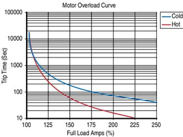
[Motor OL Hertz] defines the frequency where motor overload capacity derate should begin. The motor overload capacity is reduced when operating below [Motor OL Hertz]. For all settings of [Motor OL Hertz] other than zero, the overload capacity is reduced to 70% at an output frequency of zero.
