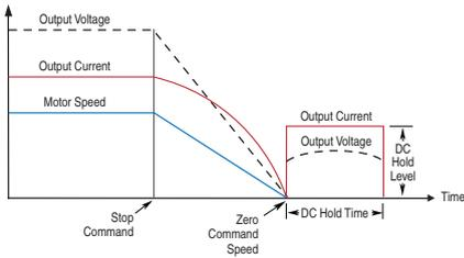
This method uses drive output reduction to stop the load.
