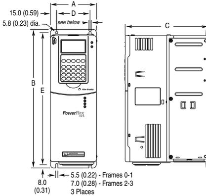
Dimensions are in millimeters and (inches).
