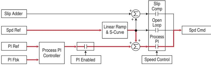
Or, it can operate as control mode by supplying the entire speed reference. This method is identified as “exclusive mode”
