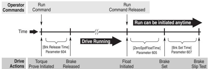
All times between Drive Actions are programmable and can be made very small (i.e. Brake Release Time can be 0.1 seconds)
