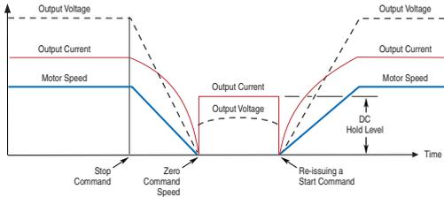
This method combines two of the methods above. It uses drive output reduction to stop the load and DC injection to hold the load at zero speed once it has stopped.
