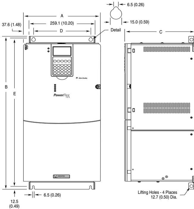
Dimensions are in millimeters and (inches).
