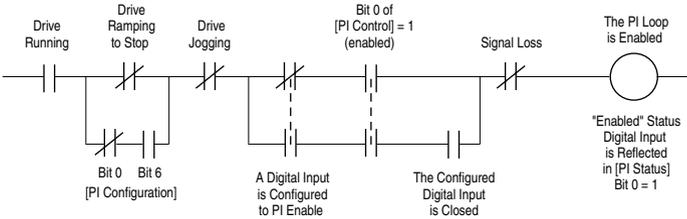
The drive must be running for the PI loop to be enabled. The loop will be disabled when the drive is ramping to a stop (unless “Stop Mode” is configured in [PI Configuration]), jogging or the signal loss protection for the analog input(s) is sensing a loss of signal.
