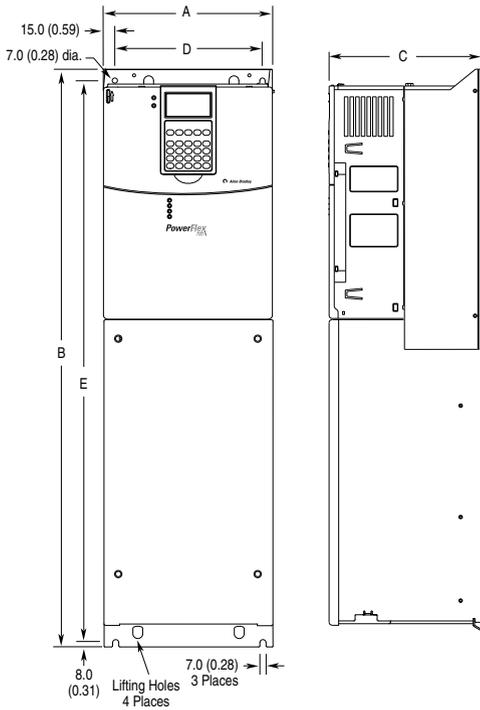
*Dimensions are in millimeters and (inches)*
