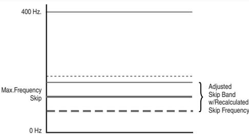
If the band is outside the limits, the skip band is inactive.
