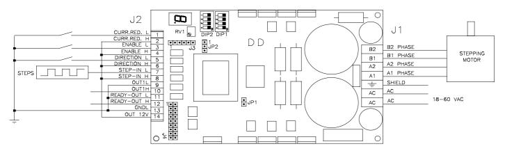
In this diagram is used internal +12V but you can use an external power supply from 12 to 24 Vdc.
