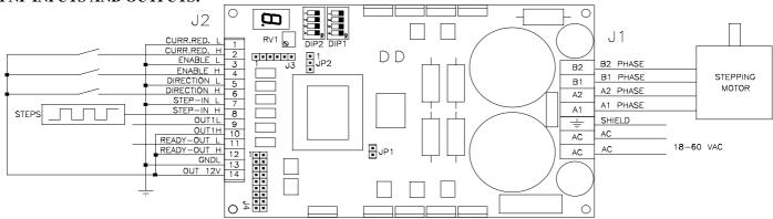
In this diagram is used internal +12V but you can use an external power supply from 12 to 24 Vdc.
