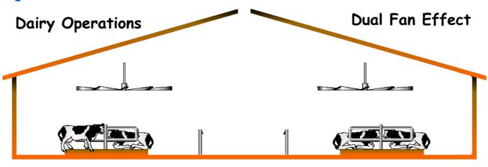
MegaFans are typically hung 16'- 18' from the floor, directly over the feed alley in a free stall barn. Although the MegaFans are available in sizes from 8 feet to 24 feet most dairies employ the 20 ft or 24 ft fan within the free stall area and 10' to 14' diameter fans in the holding pen areas.
