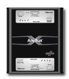
The gateway consists of two independent Ethernet interfaces, each with its own microporcessor system and TCP/IP stack.
