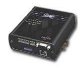
Configuration of the X-gateway is simple using BWConfig and consists of setting up an I/O table containing selected J1939 PGNs and the rate that each will be read or written from the J1939 network. BWConfig will then automatically map the I/O table to a range of addresses accessible from the X-gateway Ethernet/IP interface. The configuration is downloaded from the PC to the X-gateway via an RS232 connection and is saved in FLASH memory.
