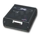
Configuration of the ABX is simple using BWConfig and consists of setting up an I/O table containing selected J1939 PGNs and the rate that each will be read or written from the J1939 network. BWConfig will then automatically map the I/O table to a range of addresses accessible from the ABX Modbus RTU interface. The configuration is downloaded from the PC to the ABX via an RS232 connection and is saved in FLASH memory.
