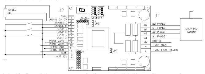
In the wiring diagram the input/output common voltage is connected to OUT 12V, you could use an external power supply from 12 to 24 Vdc for opto-isolated inputs.
