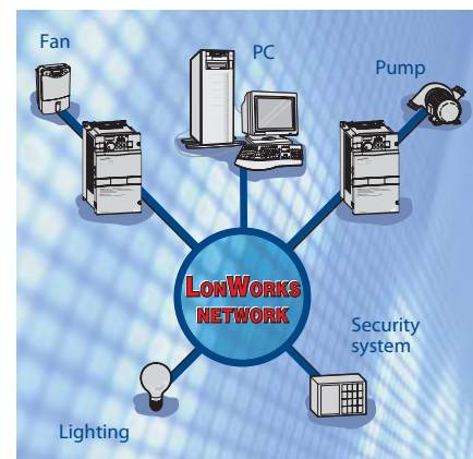
The FR-F740/F746 in a LonWorks network system
