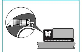
When the pressure screw is tightened to the recommended tightening torque, the steel ball seals against the spherical seat. ETP-TECHNO creates a uniform surface pressure against the shaft and hub.
