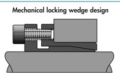
The wedge effect is augmented by the inner sleeve groove to achieve high torque transmission.
