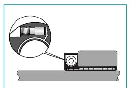
When the pressure screw is tightened to the recommended tightening torque, the piston has reached the bottom of the bore. ETP-EXPRESS creates a uniform surface pressure against the shaft and hub.
