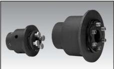
H-TLC Torque Limiters Corrosion proof design. Adjustable. Bores from .250" to 1.000". Torques from 4 to 500 in. lbs.
