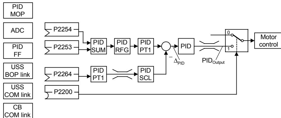
This parameter allows the user to select the source of the PID setpoint. Normally, a digital setpoint is selected either using a fixed PID setpoint or an active setpoint.
