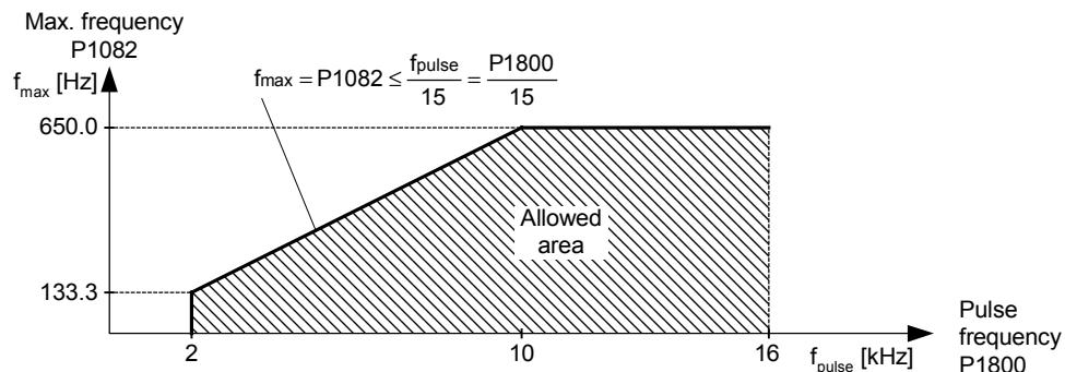
When P1300 < 20 (control mode = VF or FCC modes) then max output frequency is limited to smallest of 650 Hz or ( maximum pulse frequency / 15)
