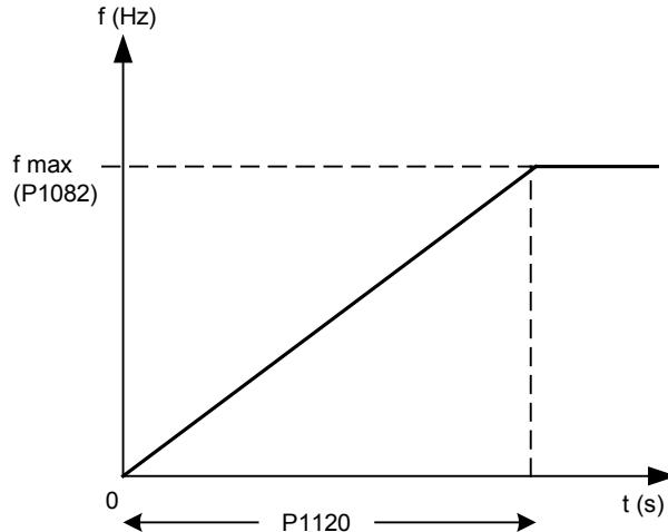
Setting the ramp-up time too short can cause the inverter to trip (overcurrent).
