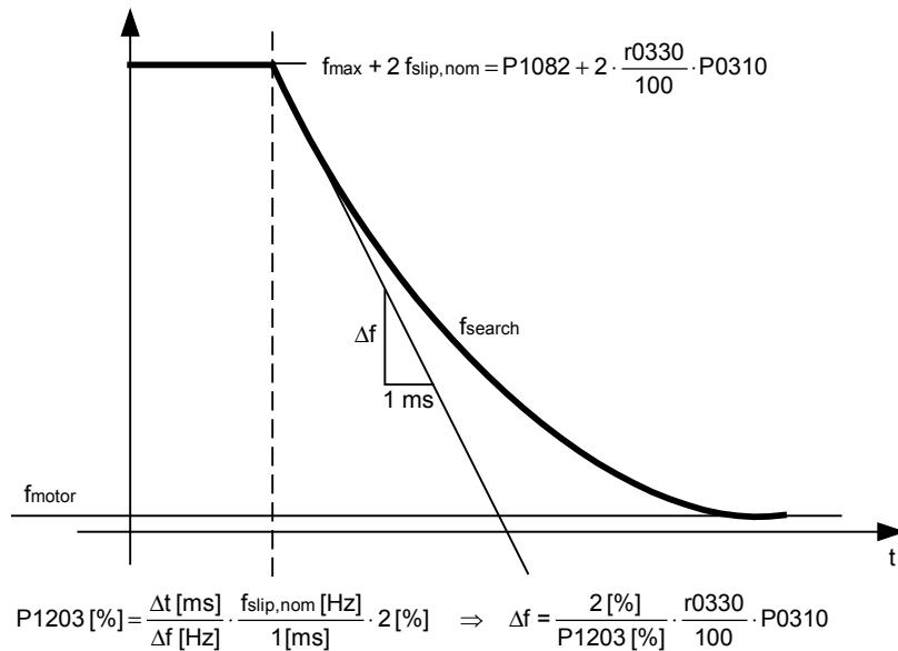
The search time is the time taken to search through all frequencies between max. frequency  $P1082 + 2 \times f_{\text{slip}}$  to 0 Hz.
