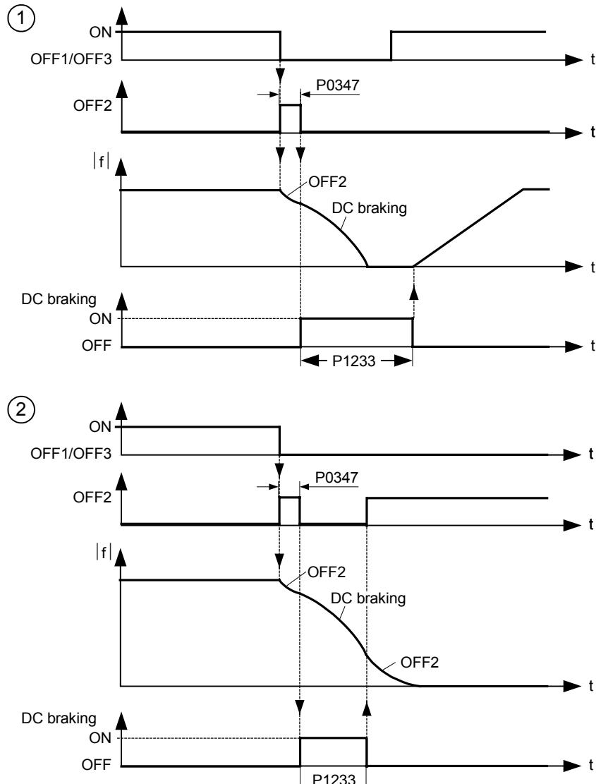
Parameter P1232 still controls the level of DC injection.
