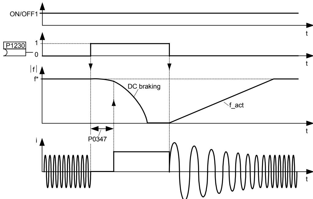
The level of DC braking is set in P1232 (DC braking current - relative to the rated motor current) which is set to 100 % by default.
