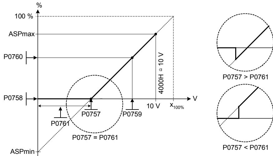
ADC value 0 to 10 V (-50 to +50 Hz):
