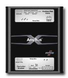
Power supply connector: 2-pole 5.08 mm Phoenix pluggable screw connector
