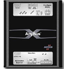
The DeviceNet Master interface can act both as a Master/Scanner and/or Adapter/Slave. The entire DeviceNet protocol is implemented into the module. The module manages control of up to 63 DeviceNet slaves. Full DeviceNet configuration can be defined and loaded into the Anybus-M module via the HMS configuration software NetTool-DN (purchased as a separate accessory) or via Rockwell's RSNetWorx.
