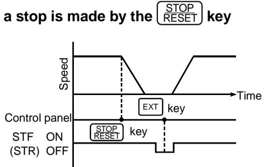
Besides the above operations, a restart can be made by performing a power-on reset or resetting the inverter with the inverter's reset terminal.
