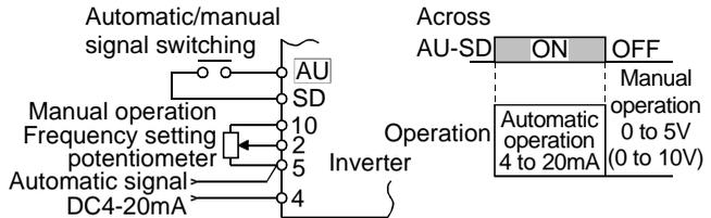
When the 4-20mADC signal is used to perform operation, always short the AU signal.
