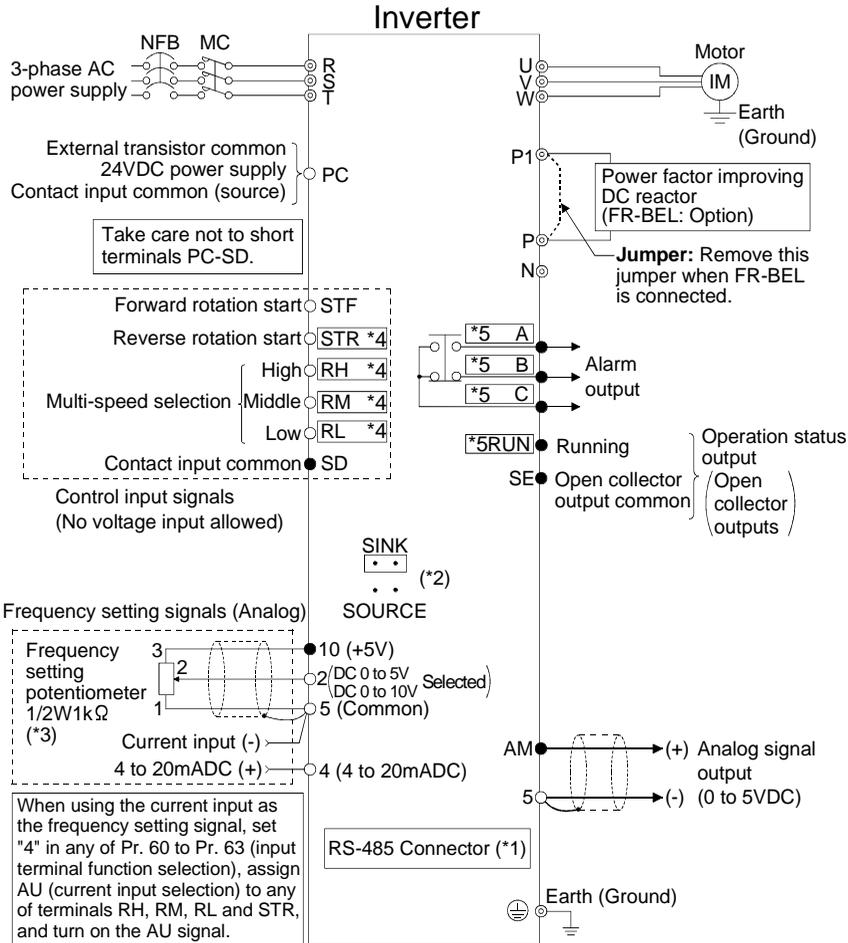
◎ Main circuit terminal ○ Control circuit input terminal ● Control circuit output terminal
