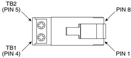
**RJ45 Adapter with Integrated Termination Resistor** –
