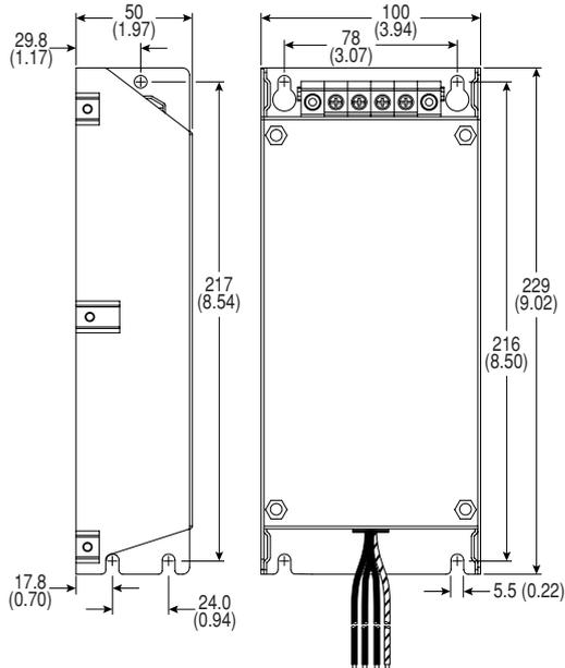
**Figure B.11 Frame C EMC Line Filters** – Dimensions are in millimeters and (inches)
