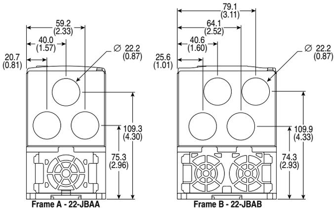
**Figure B.3 PowerFlex 4 Flange Mount Drives – Dimensions are in millimeters and (inches)**
