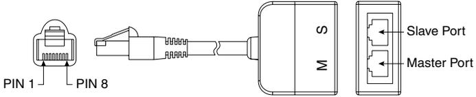
**RJ45 Two-Position Terminal Block Adapter** –
