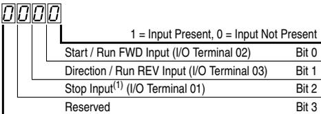
(1) The stop input must be present in order to start the drive. When this bit is a 1 the drive can be started. When this bit is a 0 the drive will stop.
