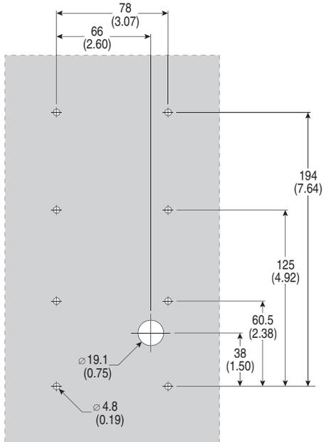
**Figure B.13 Remote (Panel Mount) Small HIM – Dimensions are in millimeters and (inches) Catalog Number: 22-HIM-C2S**
