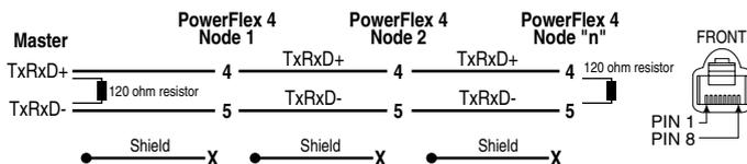
NOTE: The shield is connected at ONLY ONE end of each cable segment.
