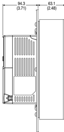
**Figure B.5 PowerFlex 4 Replacement Plate Drive Dimensions** – Dimensions are in millimeters and (inches)
