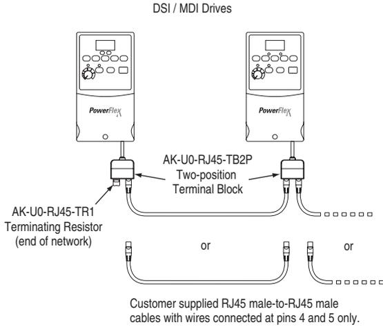
Both the Master (M) and Slave (S) ports on the RJ45 Splitter Cable operate as standard RS-485 ports in this configuration.
